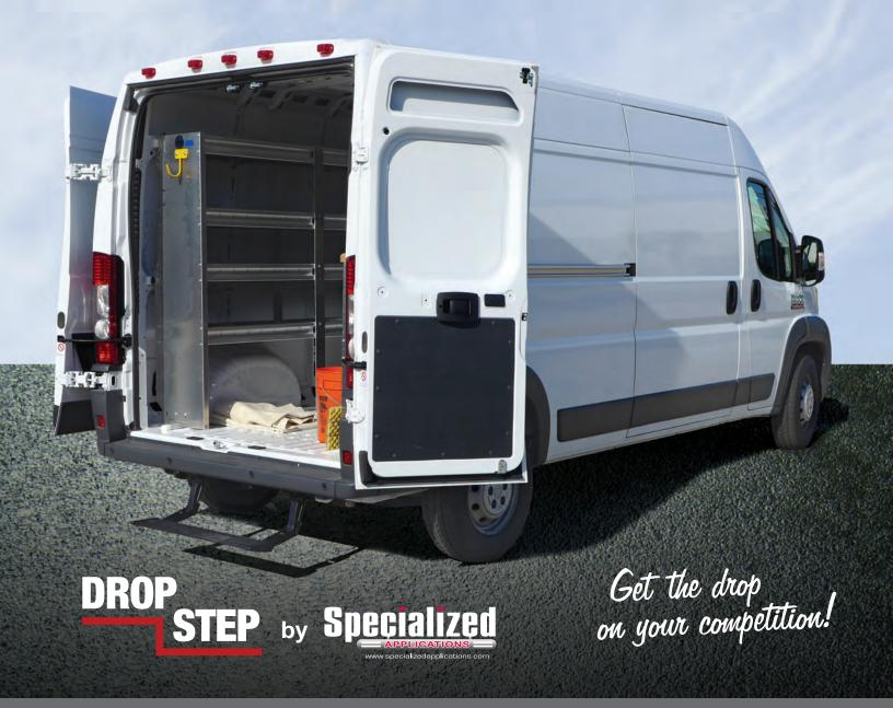
Step on to lower. Step drops down to provide improved access and safety. A nudge from your foot and the step retracts under the bumper where it stays clean and protected. Finally - problem solved for anyone who needs to get in and out of the back of their Ram ProMaster.
